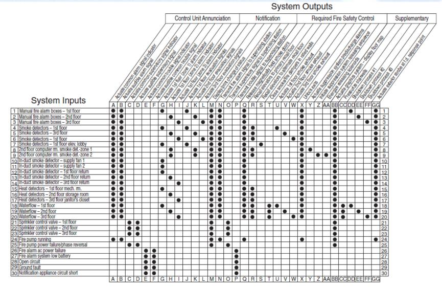
FIGURE A.14.6.2.4 Typical Input/Output Matrix.
